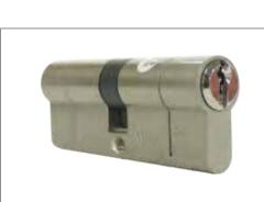
High Security Cylinder (optional extra) Superior physical strength - Cylinder design that prevents lock bumping Anti-snap now with break points allowing interior key to work even if external snap damage occurs
